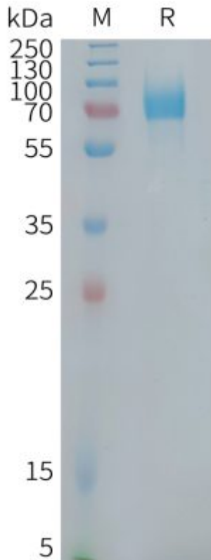
Figure 1. Human CD22(417-678) Protein, mFc Tag on SDS-PAGE under reducing condition.
